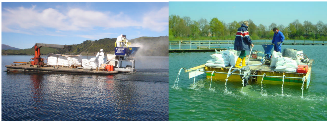
Figure 6: Phoslock® barge application on a large reservoir in New Zealand (LHS) and in a large recreational lake in the Netherlands (RHS).
