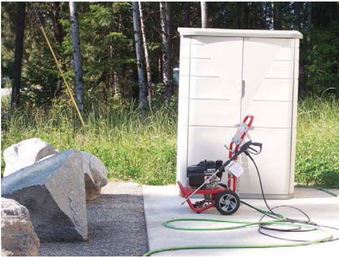
Pressure Washer for Use by Lake Host for Cleaning Watercraft and Trailers
